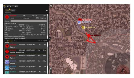
while seamlessly integrating with the existing security operations. When a drone is detected, an alarm is generated in the VMS and the drones location and pilot location are shown on a map that is output as a video stream and viewed in a VMS window, providing security personnel with a
