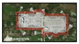
Design layout is focused on exterior fence approached with some interior coverage.
