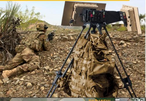
Using Advanced Detection and Classification algorithms, detecting small drones ranges from 200m to 1,000m while immediately cueing cameras to the threat. Using Web based UI (NIO) and video analytics, tighter focus is achieved and false alarms are left almost non-existent.
